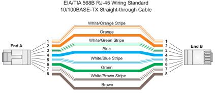
Figure B-2 Straight-through Wiring
